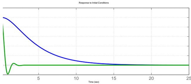
Figure 4.5: Response of the closed-loop system to initial conditions (green line) compared to the response of the open-loop system (blue line)
