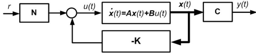
Figure 4.6: State feedback for tracking a reference input
