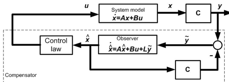
Figure 4.1: State variable compensator with observer
