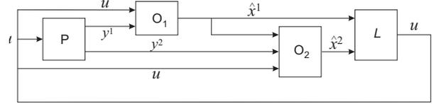
Fig. 5. Cascaded observers in closed-loop.
