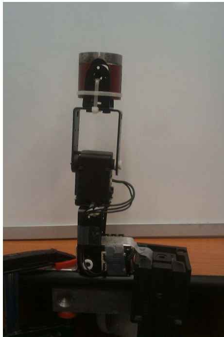
(a) A 2DOF robot arm
