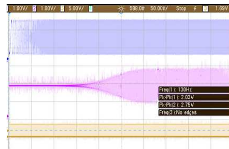
Figure 15. High-pass filter response (IIR) - hand-coded
