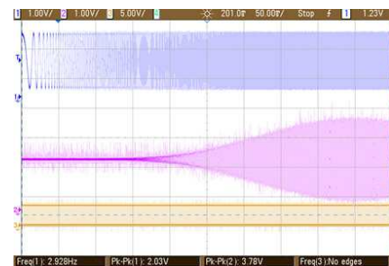
Figure 14. High-pass filter response (FIR) - hand-coded
