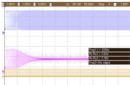
Figure 12. Low-pass filter response (IIR) - hand-coded
